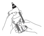
b. Insert the 9V battery into battery compartment, note the battery polarity, and then close the battery door, as shown in following figure:
